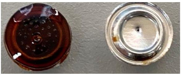
DSC sample containers for EA9396-15% acetone (left) and EA9396 (right) post testing
